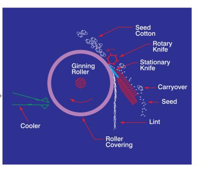
Figure 1. Principle of the rotary-knife roller gin stand. (Courtesy of the USDA-ARS Southwestern Cotton Ginning Research Laboratory.)
